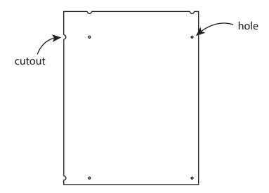
Just position cutouts on the side or end of jig against standoff barrels of the mounted plaque and mark the holes for the new plaque- repeat above. The jig can be flipped horizontally and vertically for use on top, bottom, left and right sides of previously mounted standoff plaque.
